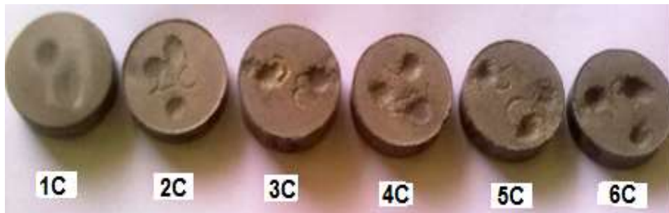
Fig. 7.1: Erosion test samples of conventionally sintered samples
