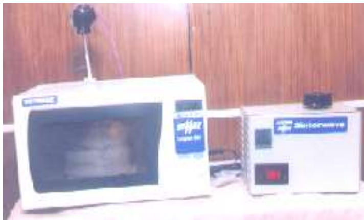
Fig. 3.8: Microwave Sintering Facility
