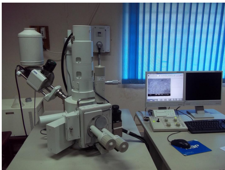
Fig. 4.8 Analytical Scanning Electron Microscope
