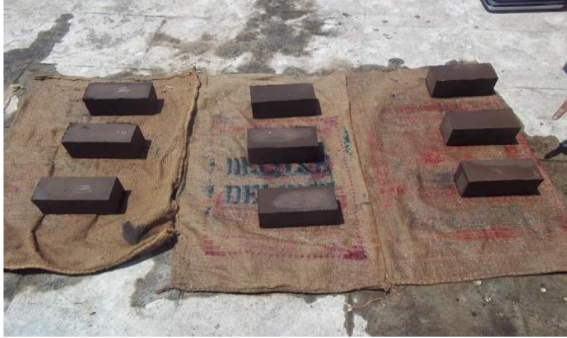
Fig. 5.14 Curing of bricks
