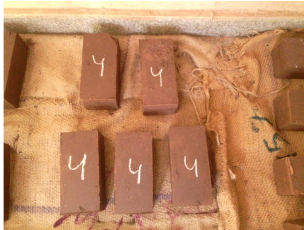
Fig. 6.77 Bricks with 65% IOW, 12.5% cement and 22.5% fly ash
