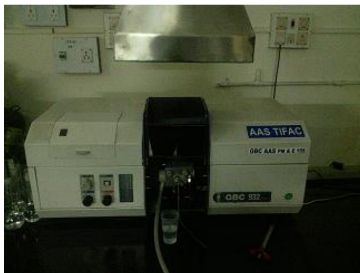
Fig. 4.10 GBC 932 Plus Atomic Absorption Spectrophotometer
