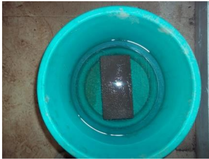
Fig. 5.15 Water Absorption Test
