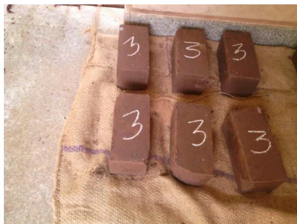
Fig. 6.58 Bricks with 65% IOW, 9% cement and 26% fly ash
