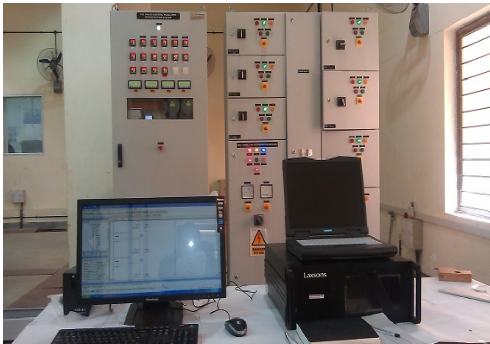
Fig.4.4: Photograph of data acquisition system of test rig
