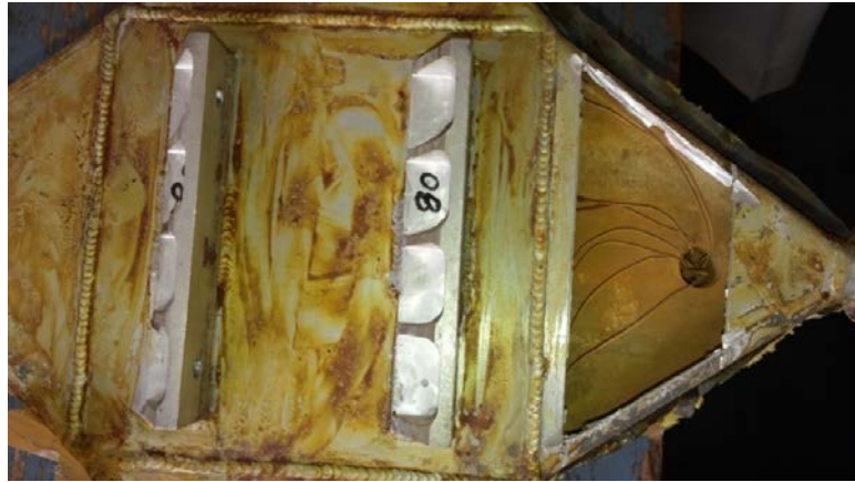
Fig. 5.3: Cut section of thermocouples inserted in test section
