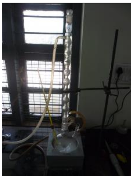
Figure 3.4 Experimental set up for the synthesis of semicarbazone intermediate
