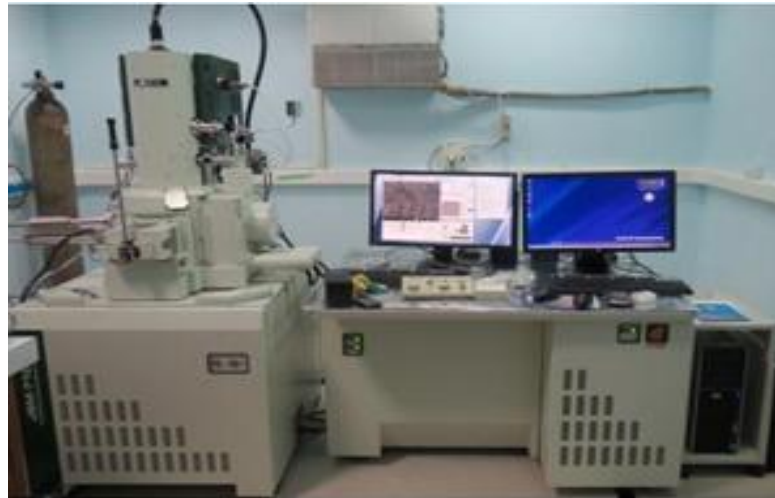
Figure 3.7. Field emission scanning electron microscope.
