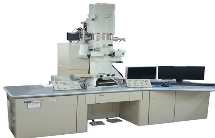
Figure 3.8. Transmission electron microscope (TEM).
