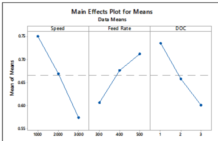
Figure 5.2: Effect of process Parameters on Surface Roughness (Ra) of AA6061
