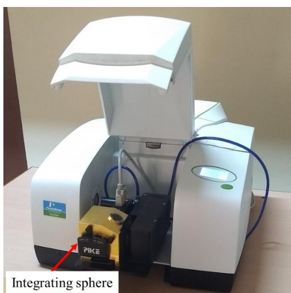
Figure 2.6: FTIR instrument with integrating sphere accessory.
