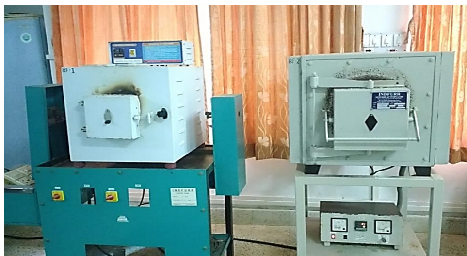
Figure 2.3: Furnaces used for glass preparation
