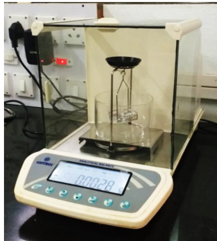
Figure 2.5: Density measurement setup used for the synthesized glasses
