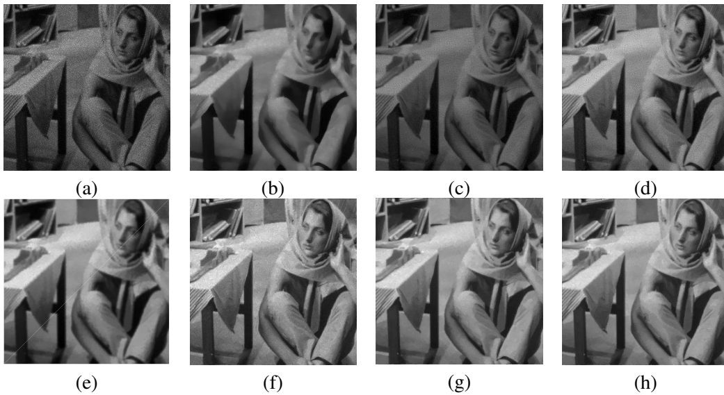
Figure 3.5 Image “Barbara” restored using various methods (multiplicative Rayleigh noise variance of input image is 0.15 and standard deviation of blurring kernel is 1.2): (a): Noisy image; images restored using (b) Model A; (c) Model B ;(d) Model C ;(e) Model D (f) Model I (g) Model II and (h) Model III
