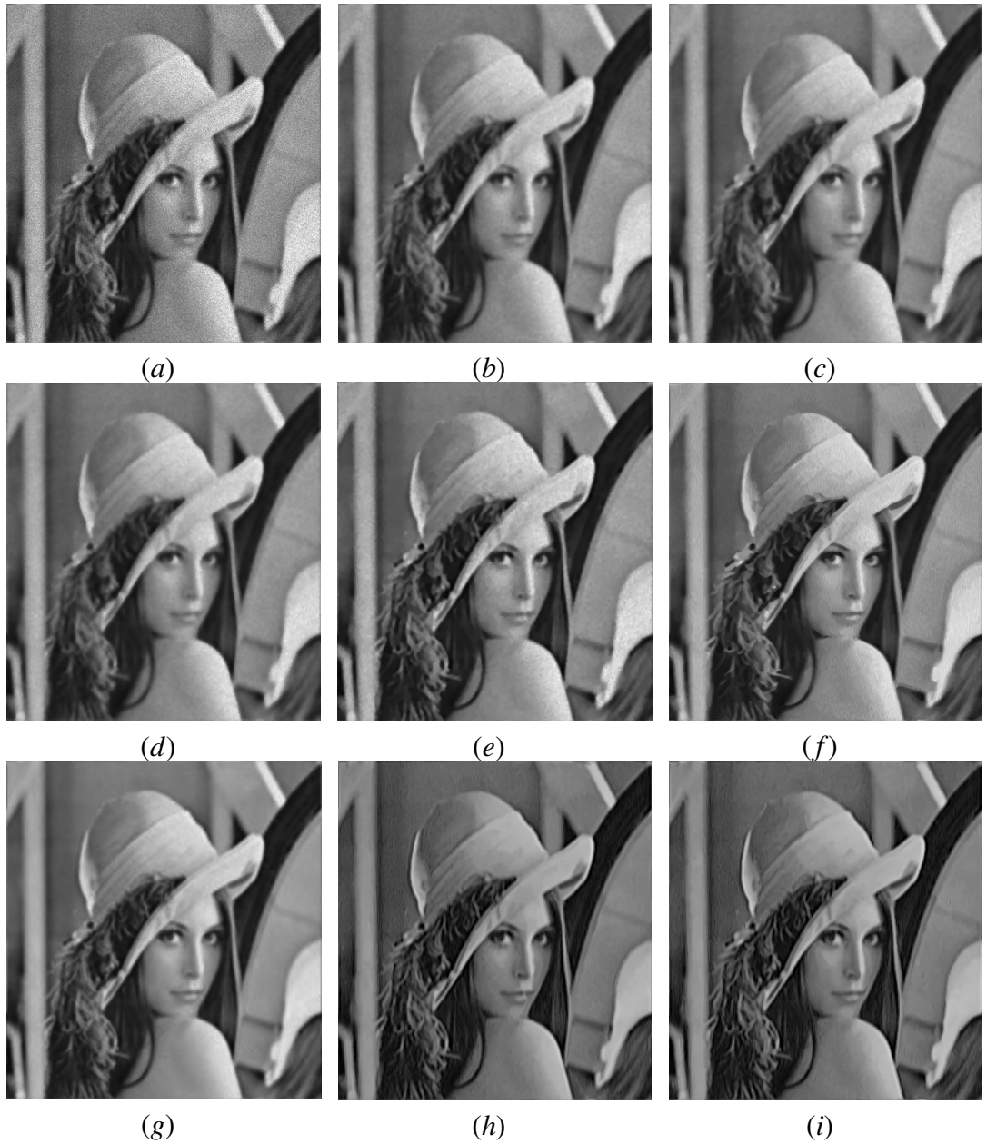
Figure 3.2 (a) Speckled and Blurred Lena image [Gamma noise variance: 0.1 and Blur kernel size: 2] (b) The restored image by SRAD method (c) The restored image by DPAD method (d) The restored image by OSRAD method (e) The restored image by AA method (f) The restored image by NLTv method (g) The restored image by BM3D method (h) The restored image by NLTv using AL method (i) The restored image by proposed method
