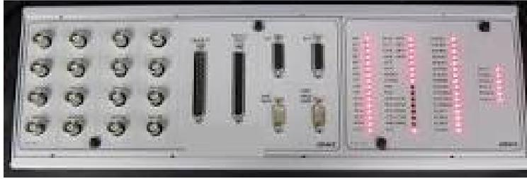
**Figure C.2:** The 19" racking system with DS1104 controller with digital I/O pins, analogue and control PWM cards
