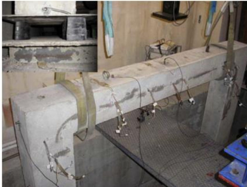
Fig. 4.17 Modal test of an RC frame: (a) In-situ modal test with spring boundary condition (top right corner). (Fang et al. 2008)
