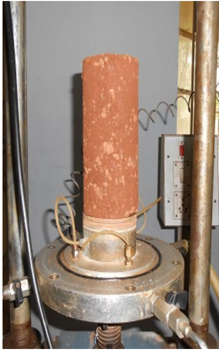
Fig.4.7a Triaxial Test Sample
