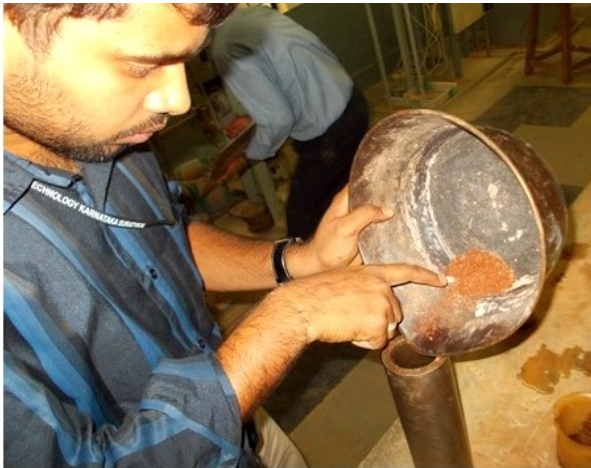
Fig. 5.4a Mixing of Dry Soil with Water
