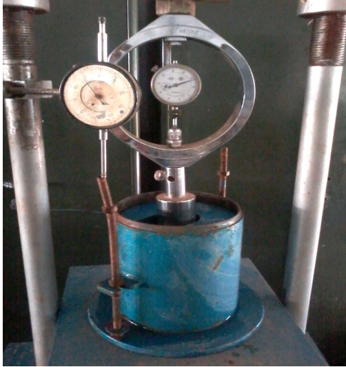
Fig.4.2k Test setup for CBR Performed in the Laboratory: Unsoaked
