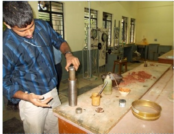
Fig. 5.4b Using the Rammer of the Kneading Compactor to Compact Soil to the Desired Density
