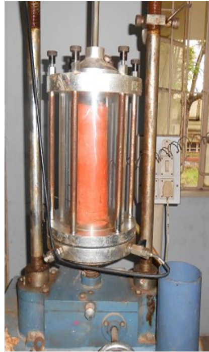
Fig.4.7b Triaxial Test Setup
