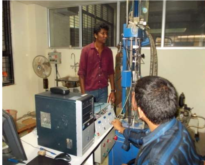
Fig. 5.5b Switch Panel for Hydraulic Pump with Cyclic Triaxial Test System
