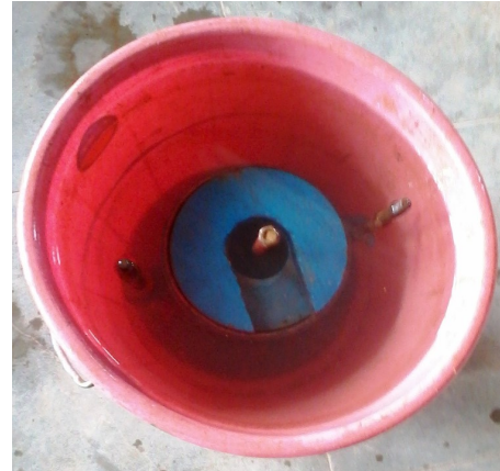
Fig.4.2l Soaking of the CBR Mould in a Bucket of Water
