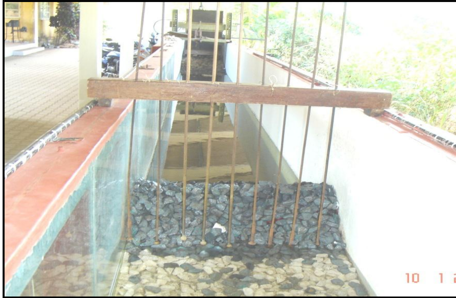
Plate 3.3 View of wave flume with profiler
