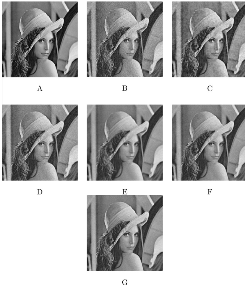
Fig. 2. Image “Lena”: (A) Original figure. (B) Blur and noisy image (out of focus blur: SNR 8 dB). (C) After applying second-order shock proposed by Alveraz et al. [14]. (D) After applying fourth-order method proposed by You and Kaveh [9]. (E) After applying fourth-order method proposed by Tai et al. [5]. (F) After applying method by Hajiaboli [22]. (G) After applying the proposed method.
