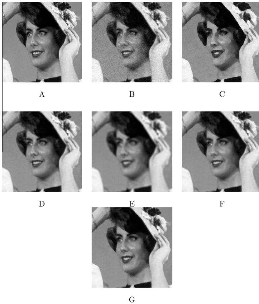
Fig. 3. Image “Woman”: (A) Original figure. (B) Blur and noisy image (out of focus blur: SNR 8 dB). (C) After applying second-order shock proposed by Alveraz et al. [14]. (D) After applying fourth-order method proposed by You and Kaveh [9]. (E) After applying fourth-order method proposed by Tai et al. [5]. (F) After applying method by Hajiaboli [22]. (G) After applying the proposed method.
