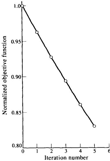
Fig. 3. Progress of optimization using SLP for trough type folded plate,
