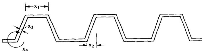
Fig. 2. Design variables for symmetrical trough type folded plate roof.
