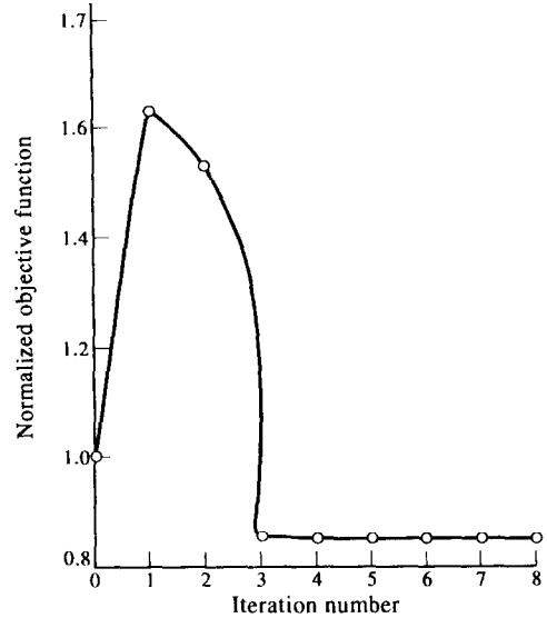
Fig. 4. Progress of optimization using SUMT for trough type folded plate.
