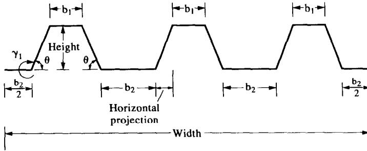
Fig. 1. Section of a trough type folded plate roof.
