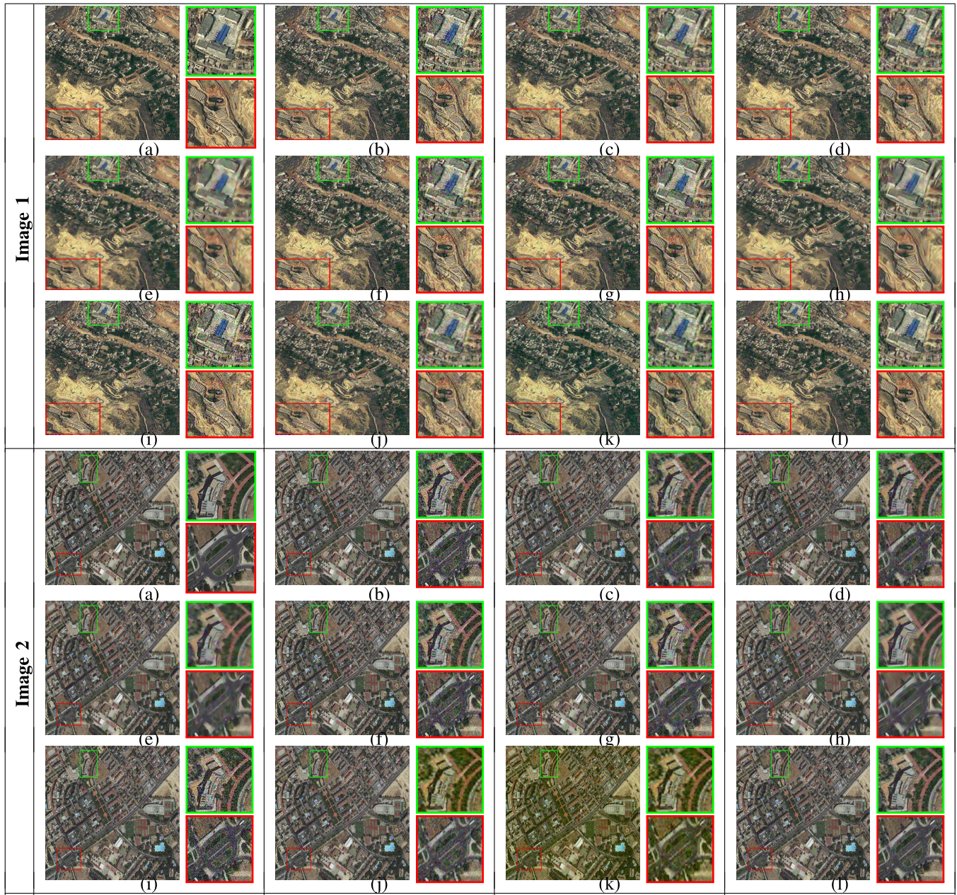
Fig. 3. Simulation results of denoising Images 1 and 2 corrupted with Gaussian noise of variance 30% using state-of-the-art denoising algorithms. (a) Original. (b) Noisy. (c) 2-D-NLMS. (d) 2-D-APA. (e) BM3-D-PCA. (f) PDE-AIP. (g) CII-NLM. (h) DST. (i) SSTV. (j) 2-D ABC adaptive filtering. (k) JADE. (l) Proposed ACSWF.
