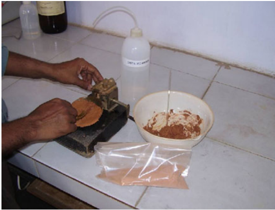
Fig. 3 Liquid limit test in the laboratory
