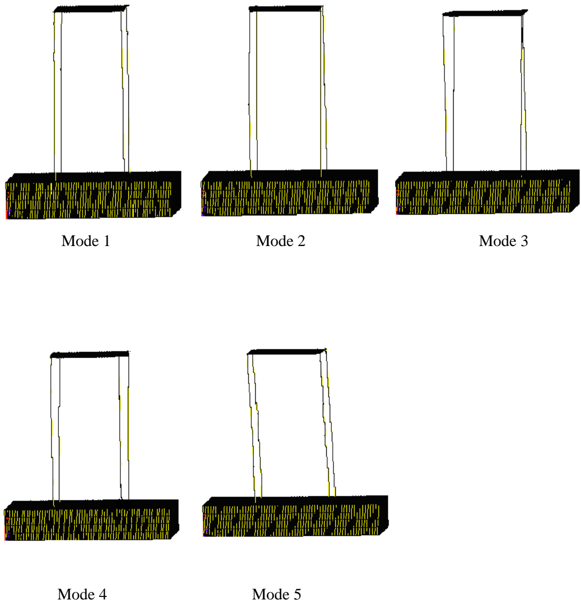
Fig 4.5 Mode shapes of simplified berthing structure with soil mass
